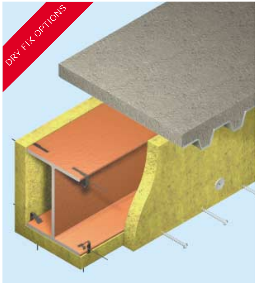
The unique Rockwool Conlit 150 dry fix clip system (International Patent Application No PCI/GB 00/01955)
